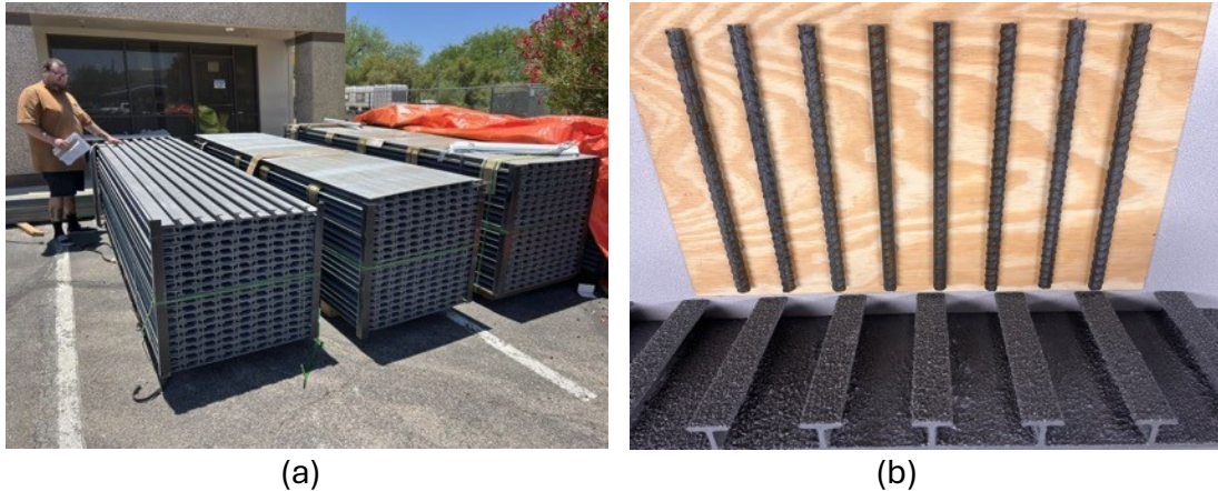
Fig. 2. T-panels: (a) 3-ft wide x 12 or 18-ft long; (b) close view of grit coated surface and equivalency to steel reinforcing bars.
