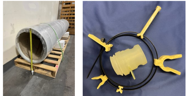
Fig. 1: A roll of FLF and samples of spacers, rebar holders and grout injection port
