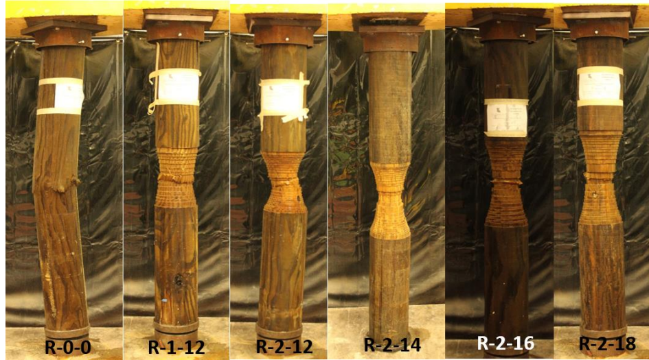
Figure 12: Testing of undamaged and damaged-unrepaired timber piles loaded concentrically
