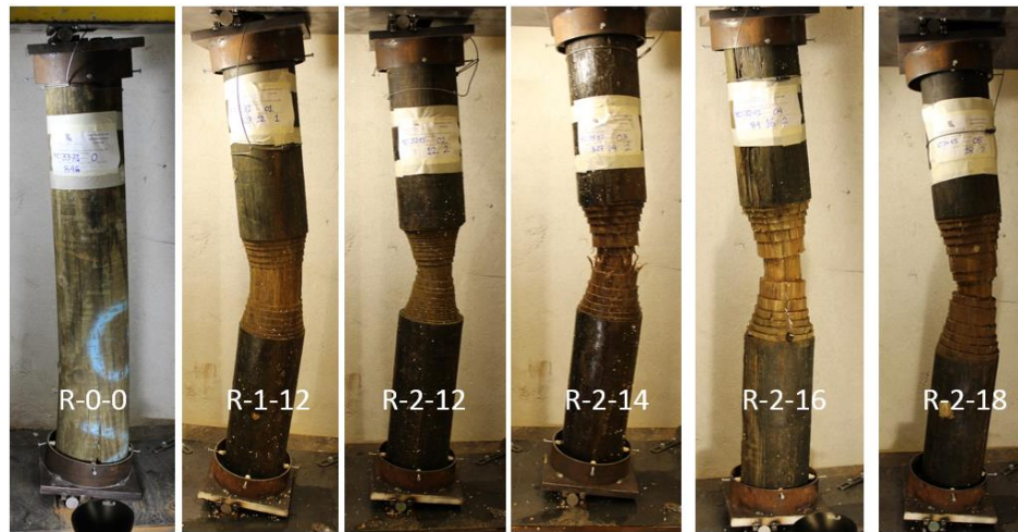
Figure 25. Testing of undamaged and damaged-unrepaired piles loaded eccentrically
