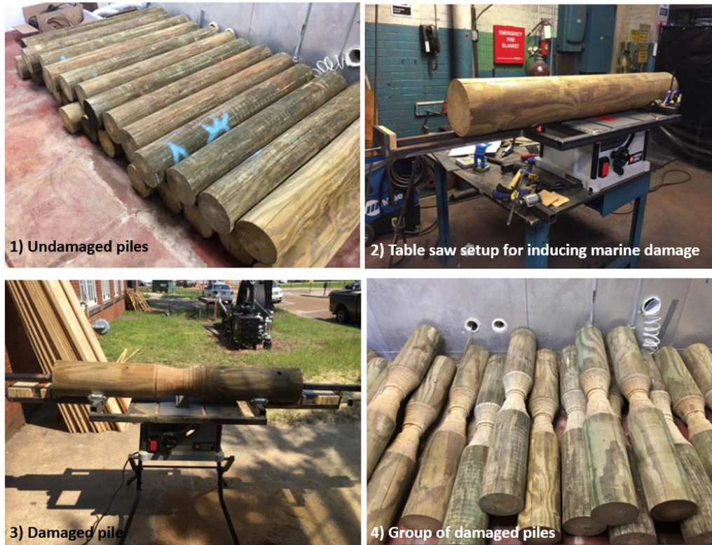
Figure 4. a) Undamaged piles, b) setup for inducing marine damage, c) damaged single pile, d) damaged group of piles
