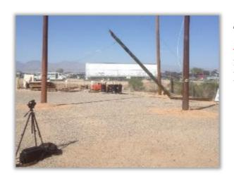
This time, the pole failed at a load of **3,200 pounds** and at a point 2-feet 9-inches below ground where the PileMedic<sup>TM</sup> jacket was terminated.
