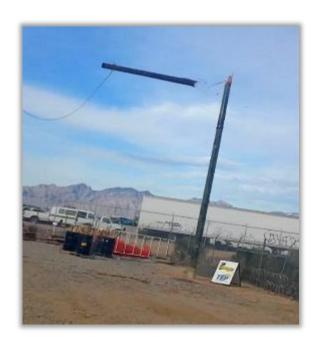
The strengthened pole was tested and it broke at a load of 2,400 pounds, exactly at the point where the repair had stopped.
