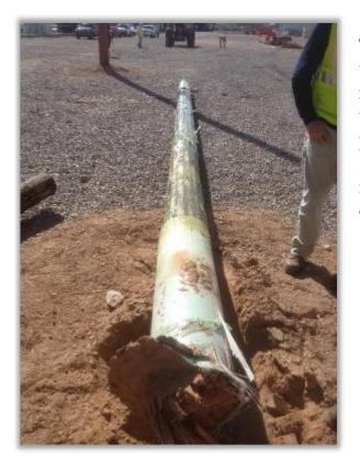
The 28.5 feet long portion of the pole that was wrapped with PileMedic<sup>TM</sup> remains undamaged and is shown in this photograph. We plan to test this piece as a simply-supported beam subjected to a concentrated load at midspan to determine its flexural capacity.
