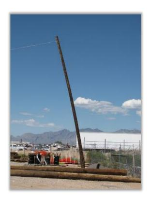
A Class III 45ft- wood distribution pole was tested in the field.
