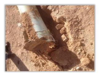
The end of the broken pole is shown here.
