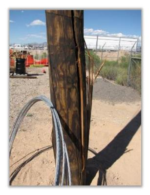
The pole broke at approximately 5 feet above ground at a load of **1,070 pounds.**
