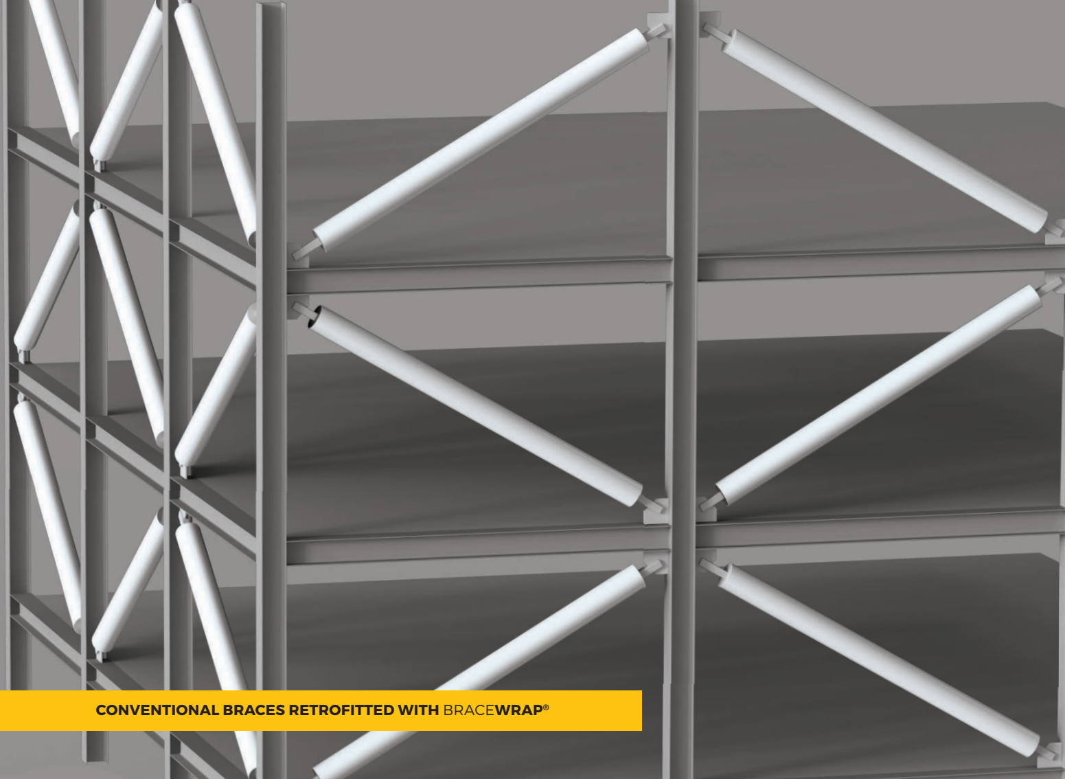
Comparison of Conventional Braced Frames (CBF) and Buckling Restrained Braced Frames (BRBF)
