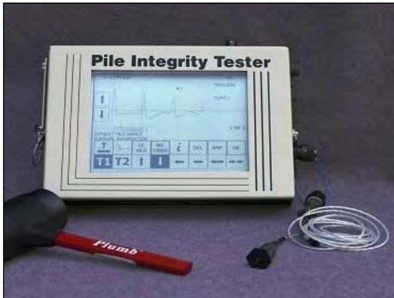
Figure 9.21. Equipment used in Pile Integrity Testing
