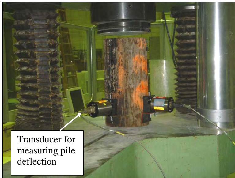
Figure 5.9. Pile compression test
