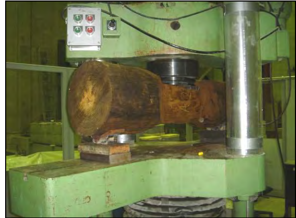
(b) Control pile section – bending
