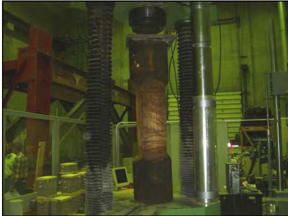
(a) Control pile section – axial
