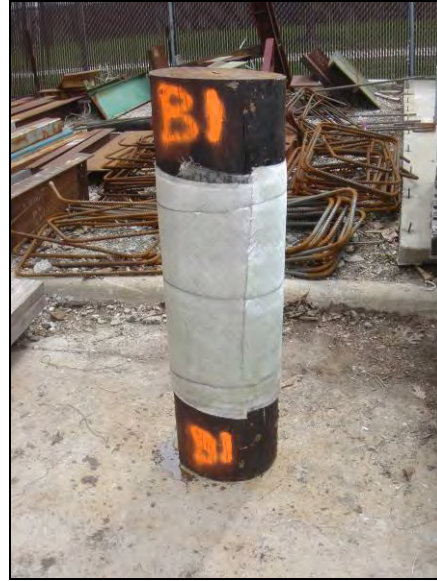
(b) Pile subjected to axial loading
