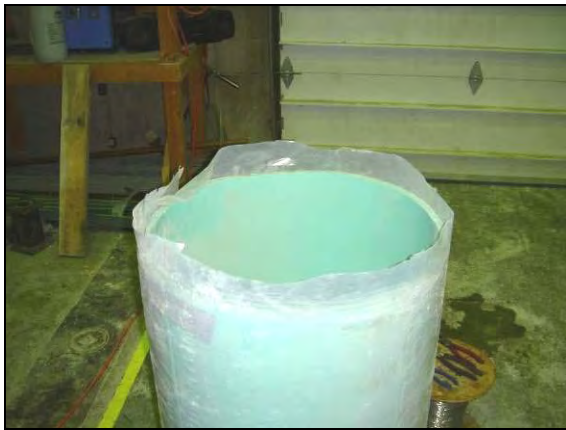
(a) PVC pipe used as a shell mold
