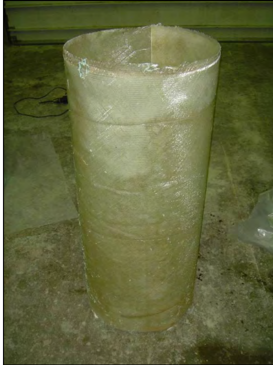
Figure 13.13. FRP shell detached from PVC pipe after curing for three days
