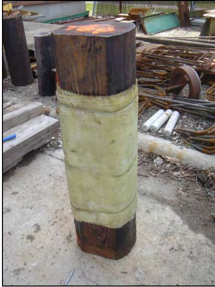
(a) Pile subjected to flexural loading
