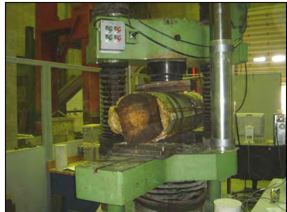
(f) Repair method C – bending
