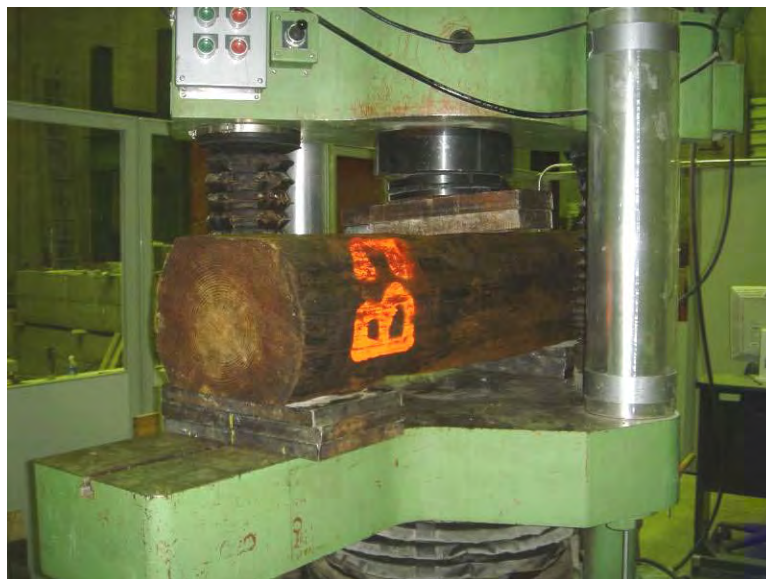
Figure 13.3. Pile sides flattened for conducting bending tests
