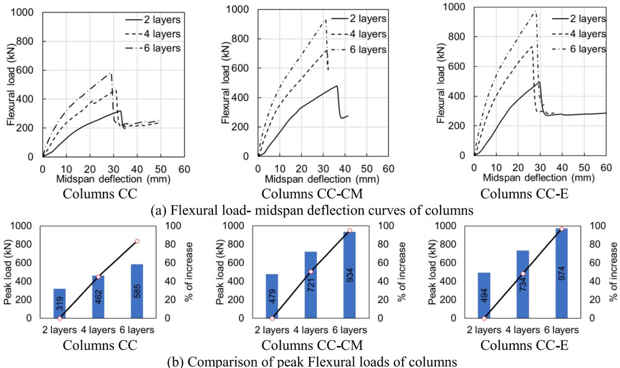
**Fig. 20.** Influence of GFRP thickness.
