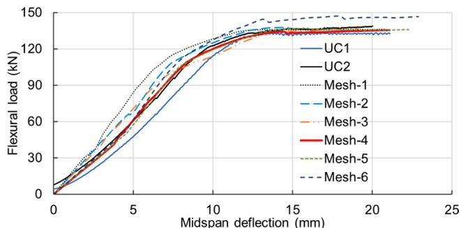
Fig. 13. Mesh sensitivity analysis.
