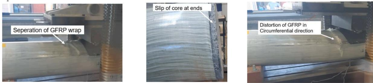
Fig. 7. Failure mode of column CC2.
