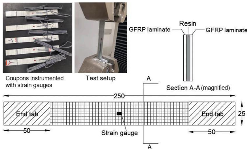
(a) Test setup and details of tensile coupons (all dimensions in mm)
