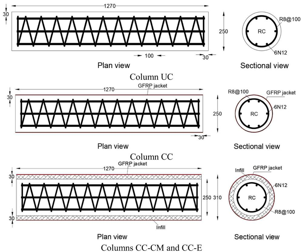
Fig. 2. Plan and sectional views of tested columns (all dimensions in mm).
