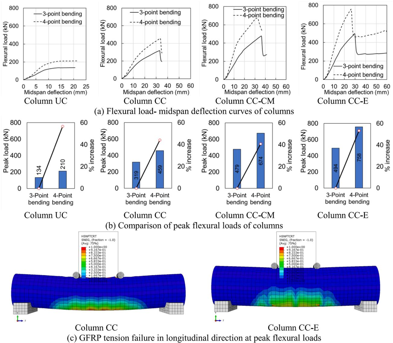
Fig. 22. Influence of variation the loading from three-point to four-point bending.
