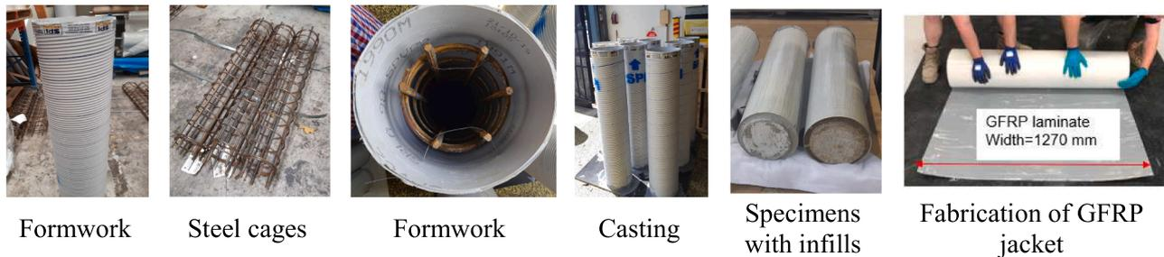
Fig. 3. Preparation of full-scale columns.
