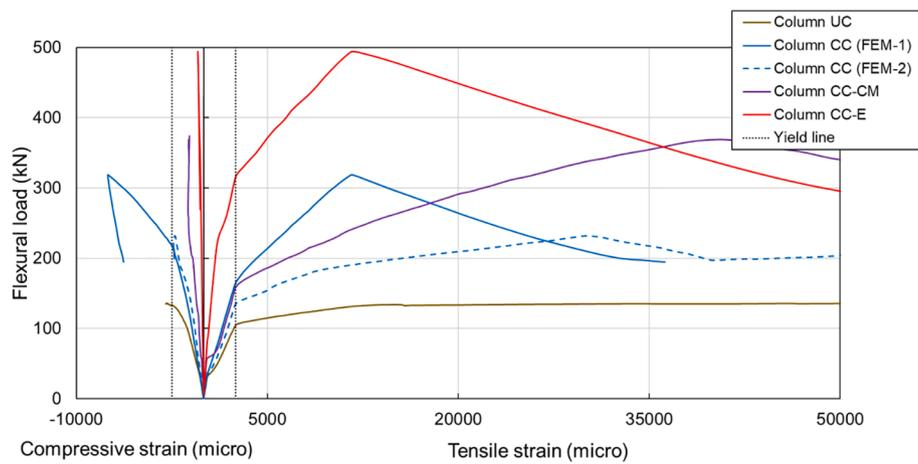
Fig. 15. Predicted flexural load-strain behaviour of longitudinal steel bars at midspan.
