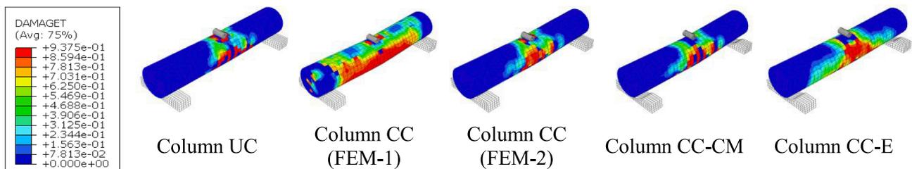
Fig. 16. Tensile damage in concrete at peak flexural loads.
