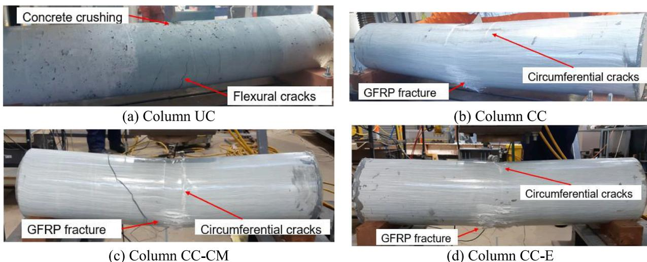
Fig. 6. Failure modes of columns tested under flexure.
