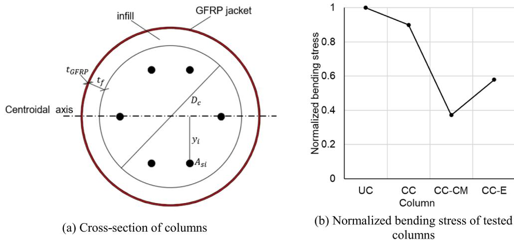
Fig. 10. Effect of enlarged sections due to GFRP wrapping system.
