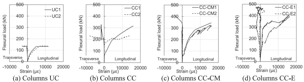
Fig. 11. Experimental flexural load-strain curves of the tested columns.
