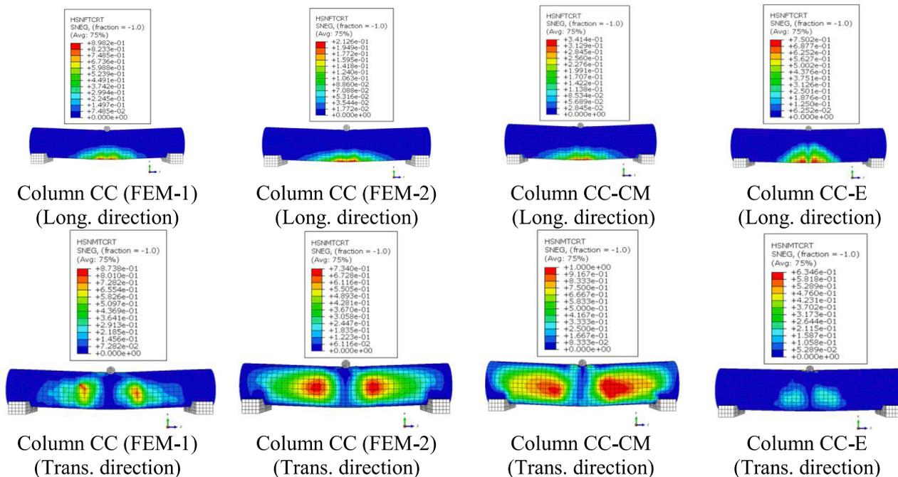
Fig. 18. GFRP tension failure in longitudinal and transverse directions at peak flexural loads.
