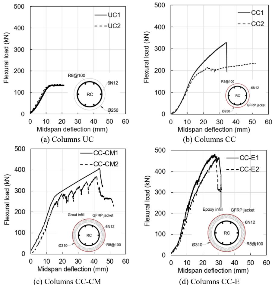
Fig. 8. Experimental load- midspan deflection curves of tested columns\*. \* Note: All dimensions in columns’ cross sections are in mm.
