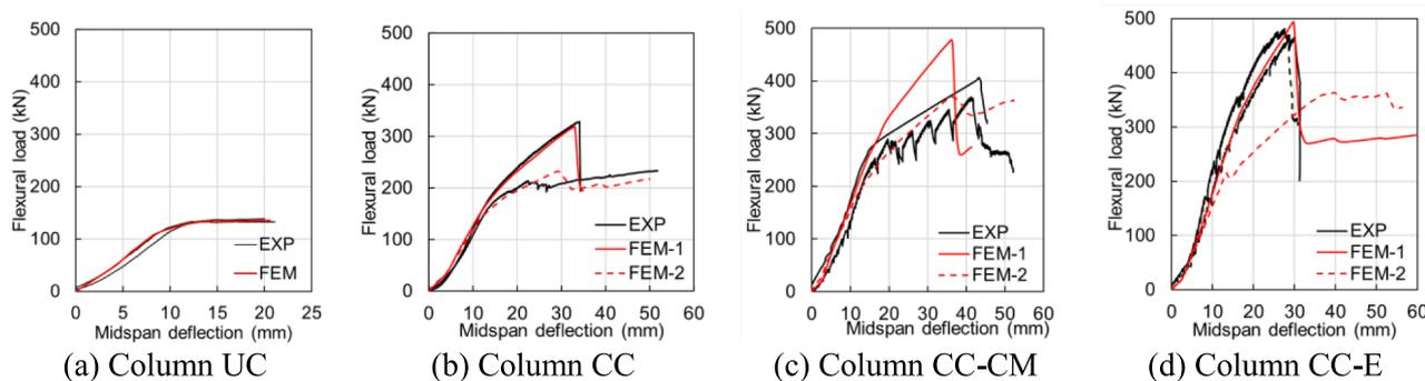
Fig. 14. Experimental and FEM flexural load- midspan deflection curves.
