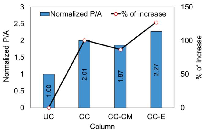
Fig. 9. Normalized P/A of tested columns and corresponding percentage of increase.
