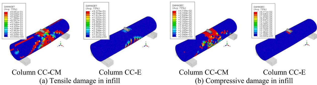
Fig. 17. Tensile and compressive damage in infills at peak flexural loads.
