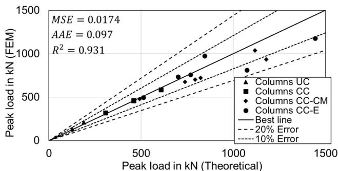
Fig. 23. Comparison between FEM and theoretical results for the peak flexural loads.
