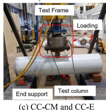
Fig. 4. Test setup of full-scale columns.
