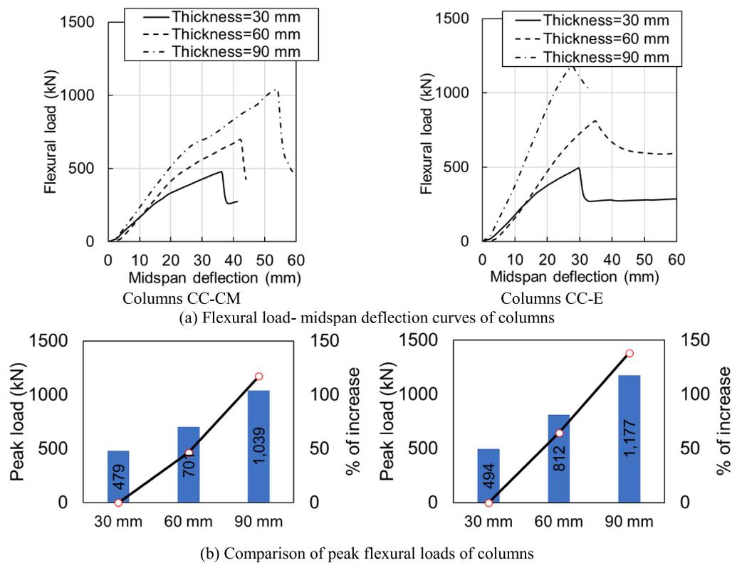
Fig. 21. Influence of infill thickness.
