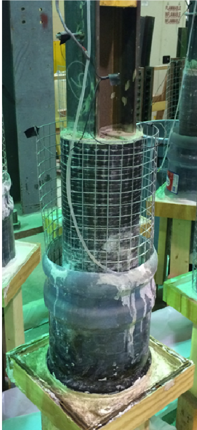
Figure 10.43: A damaged pile repaired with Repair System 2 (S2-12-Cor) showing no evidence of corrosion
