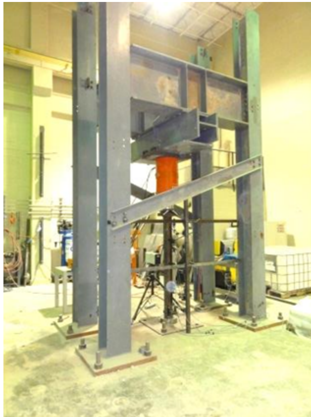
Figure 10.22: Loading frame for failure testing of the test piles
