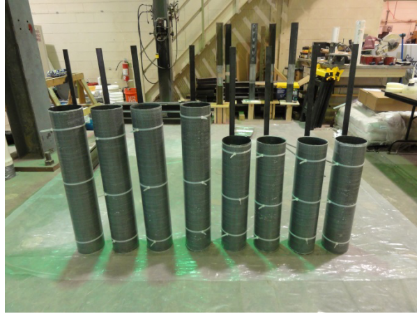
Figure 10.11: Fabricated FRP jackets for Repair System 1
