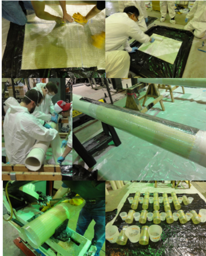
Figure 10.13: Fabrication of cylindrical GFRP shells
