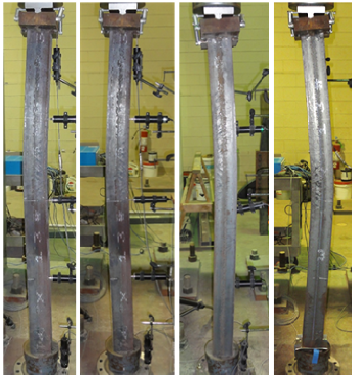
Figure 10.25: Failure of an undamaged control column (CONTs)
