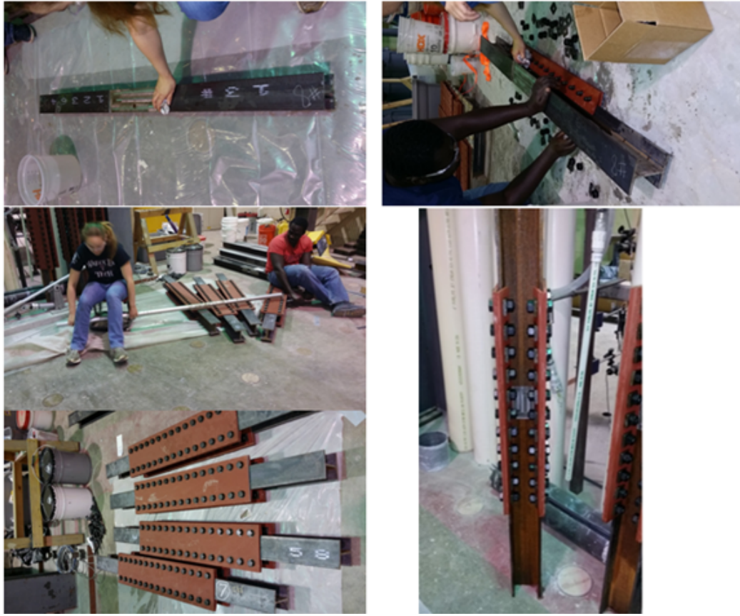
Figure 10.17: Fabrication of Repair System 3
