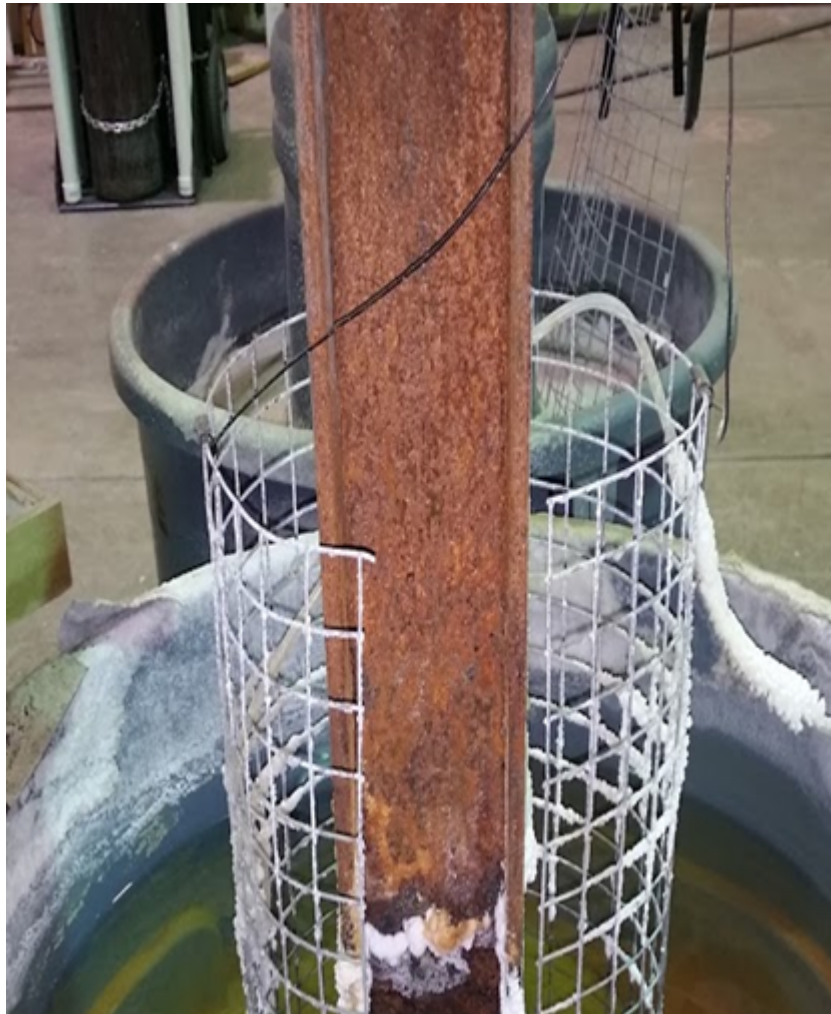
Figure 10.41: Undamaged pile (CONT-Cor) showing the rust build-up
