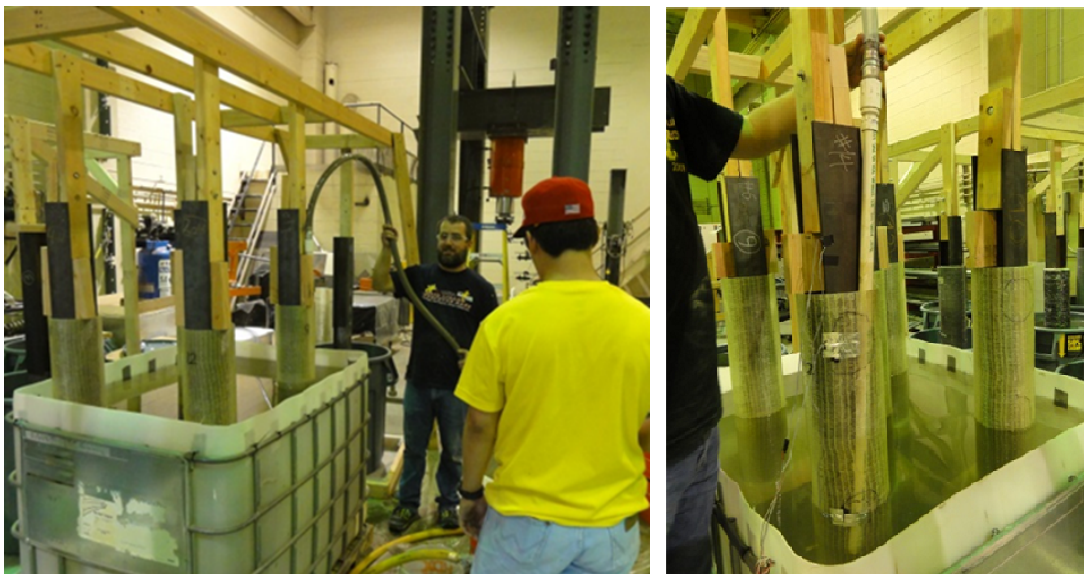
Figure 10.15: Grout injection into the voids between the GFRP shell and the pile
