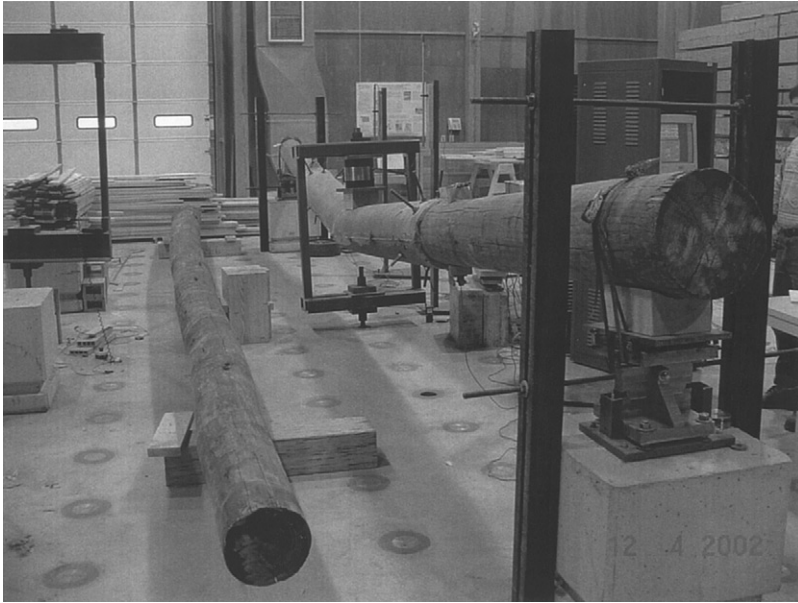
Fig. 3. Test set-up for repair system C.
