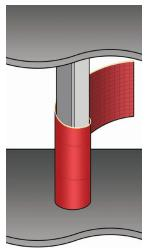
Figure 4: Square concrete columns wrapped in a continuous band of super laminate to form a cylindrical structural jacket.
