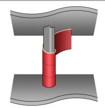
Figure 5: Steel column encased in a cylindrical seamless structural jacket constructed with super laminate.
