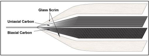
Figure 2: Various layers of fabric can be incorporated into a single sheet of super laminate.
