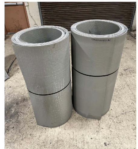
Fig. 1: FRP laminates made of sheets of carbon or glass fabric up to 9 ft wide, saturated with resin and passed through a press
