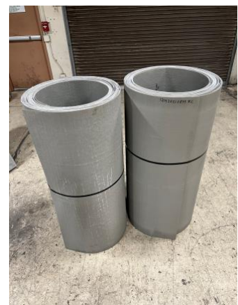
Fig. 2. PileMedic® laminates coiled in 4-foot-wide rolls for shipment.
