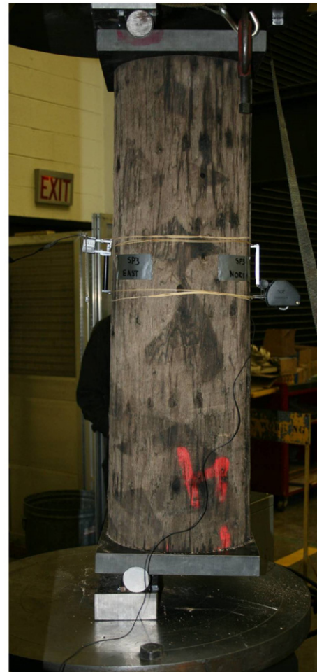
Fig. 4. Compression–flexure test setup and instrumentation.
