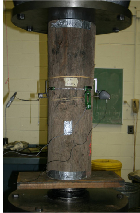
Fig. 3. Compression test setup and instrumentation.
