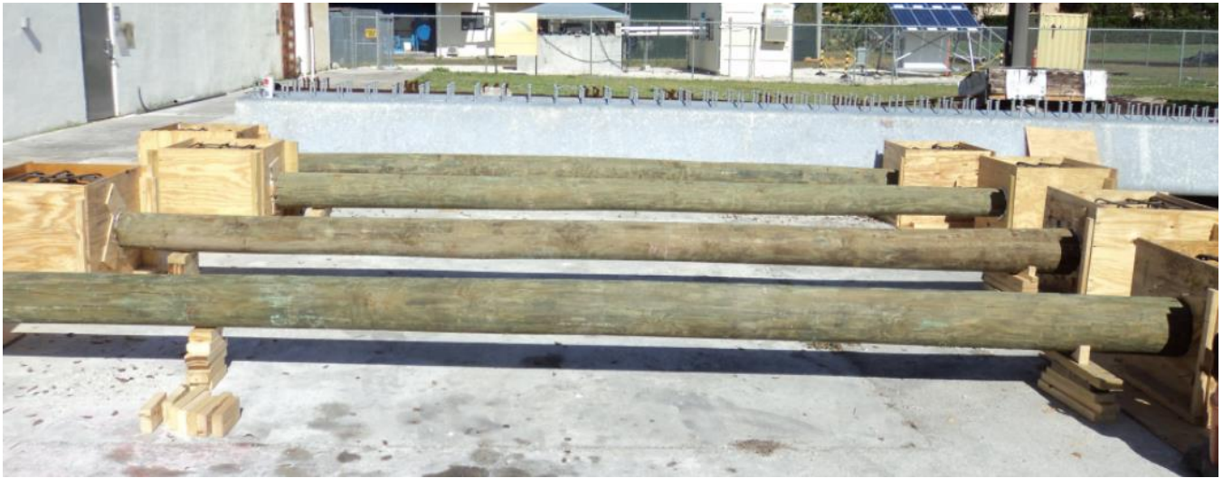
Figure 5.1: Full Scale timber pile test specimens
