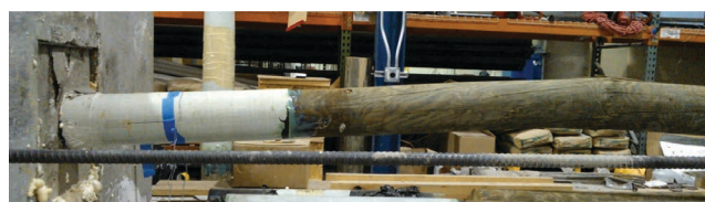
FIGURE 8 Failure of Specimen 4 (damage 2-in. deep filled with grout).
