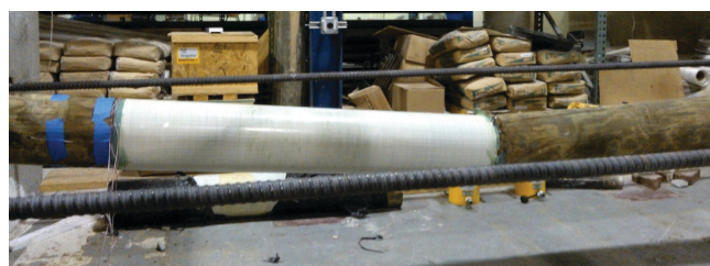
FIGURE 7 Failure of Specimen 3 (damage 2-in. deep filled with grout).
