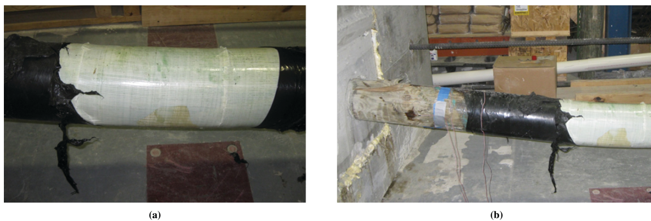
FIGURE 6 Failure of Specimen 2 (damage 1.5-in. deep filled with resin).
