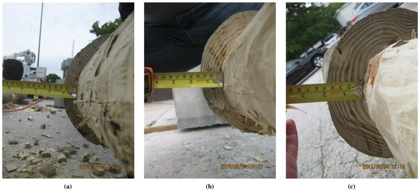
FIGURE 2 Damage in timber pile test specimens: (a) 1-in. deep, (b) 1.5-in. deep, and (c) 2-in. deep.
