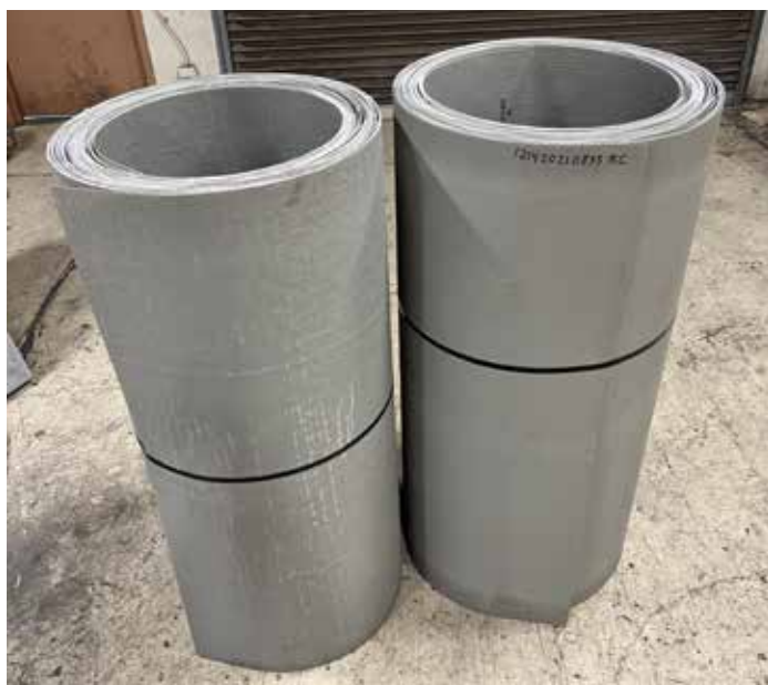
Figure 2. PileMedic laminates coiled in 4-foot-wide rolls for shipment.
