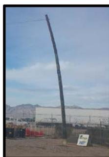
*Repaired pole was tested and failed at a load of 2,400 pounds!*
