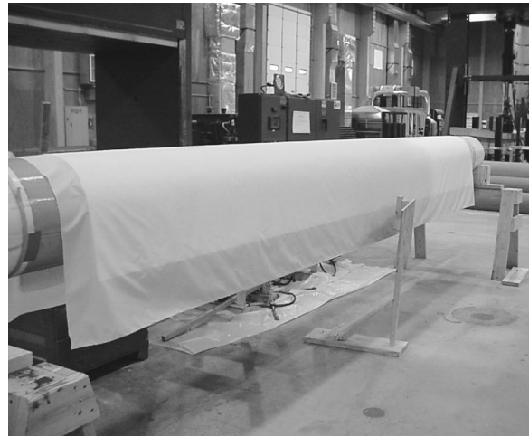
Fig. 8. Dry fabrics and peel ply on PVC mold
