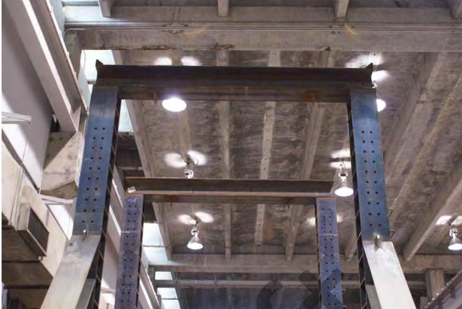
Figure 17. Stabilizer beams on top of the supports
