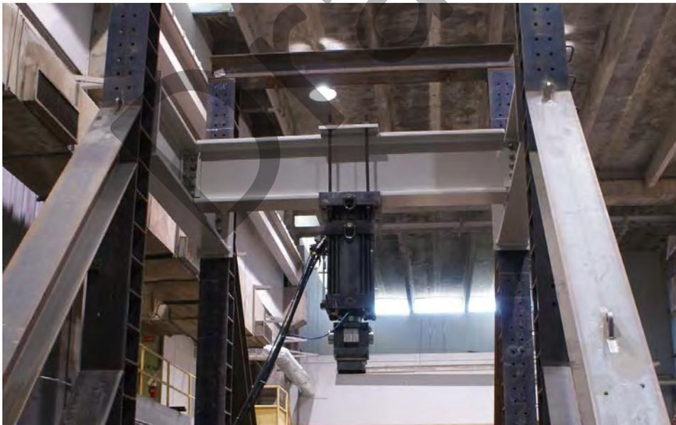
Figure 18. Loading beams installed with actuator
