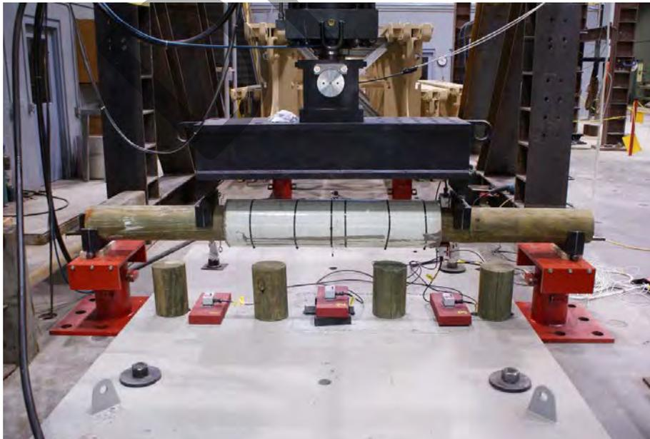
Figure 60. T-RD-2 timber specimen prior to flexural testing
