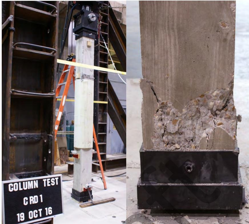
Figure 52. C-RD-1; left: prior to testing, right: end crushing of column after load testing
