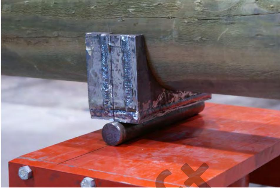
Figure 30. End roller support for timber beams
