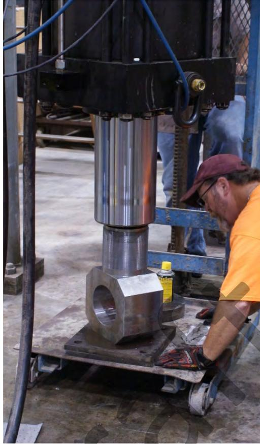
Figure 22. Load pin clevis eye threaded into hydraulic actuator end
