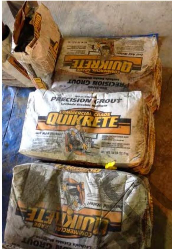
Figure 9. A commercial, non-shrink grout product was used
