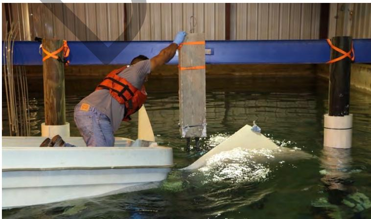
Figure 2. ERDC divers train on wrap installation in the flooded sump
