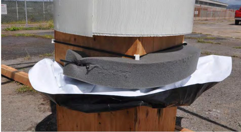
Figure 8. FRP jacket lifted to reveal foam insert and skirt
