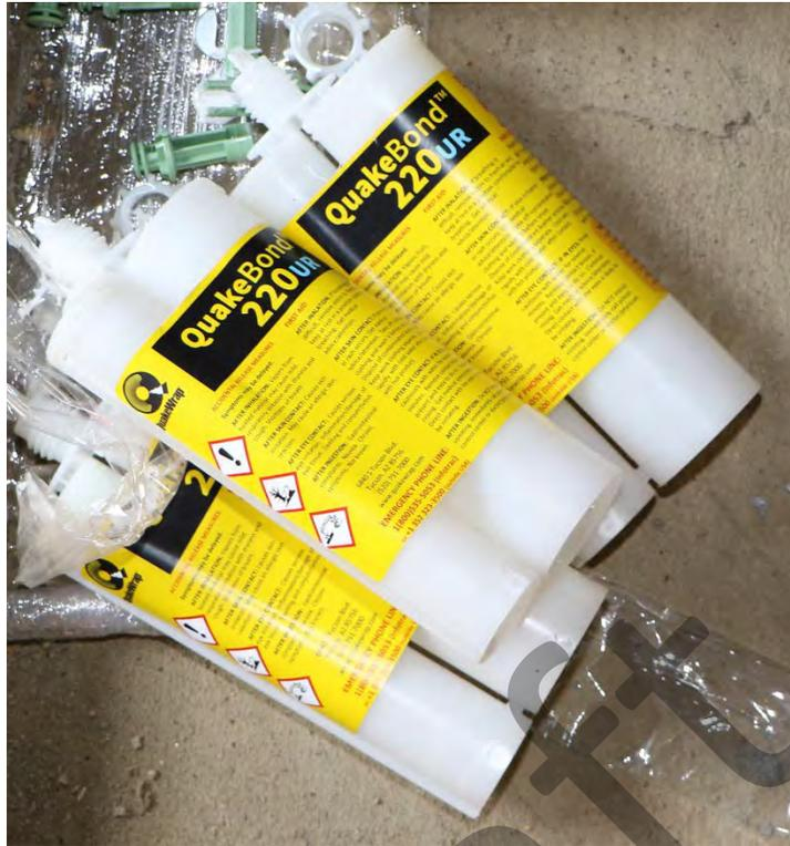
Figure 5. Two-part epoxy adhesive used to bond FRP wraps
