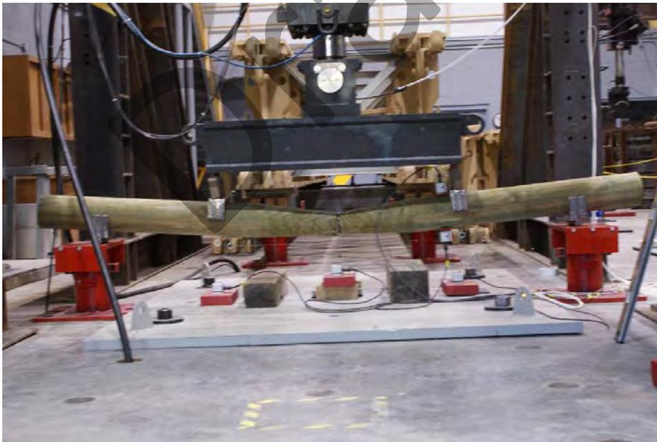
Figure 58. Typical tapered timber specimen after flexural testing
