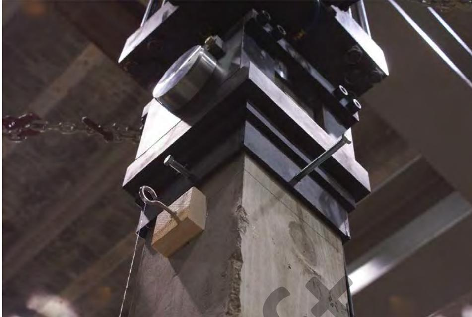
Figure 24. Upper column end cap for concrete column installed beneath load pin clevis and actuator
