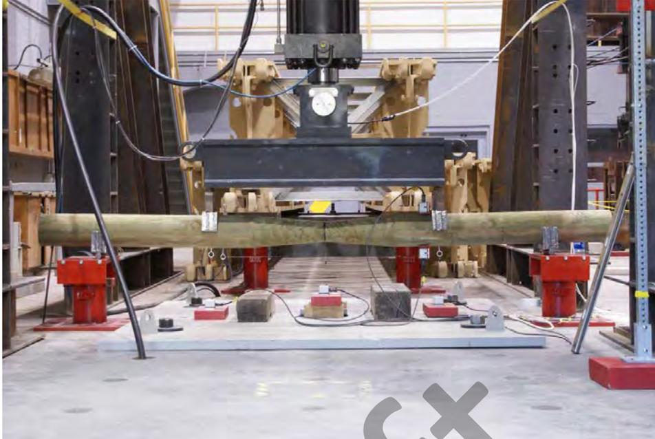
Figure 57. Typical tapered timber specimen prior to flexural testing
