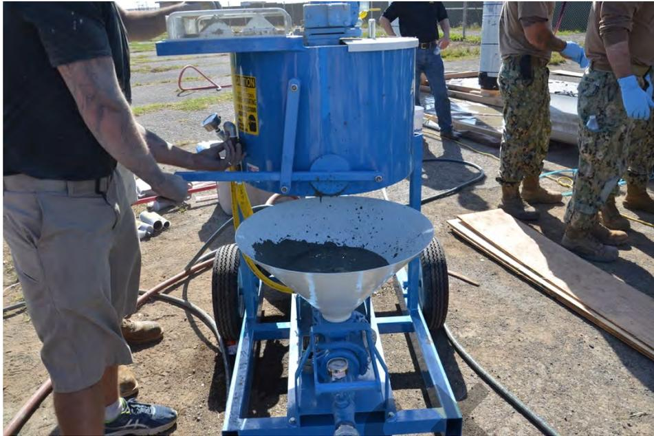
Figure 81. Air-powered grout pump
