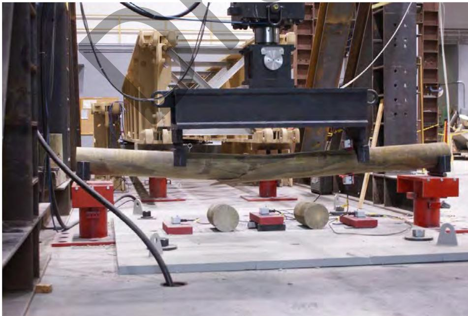
Figure 55. Typical timber control specimen after flexural testing
