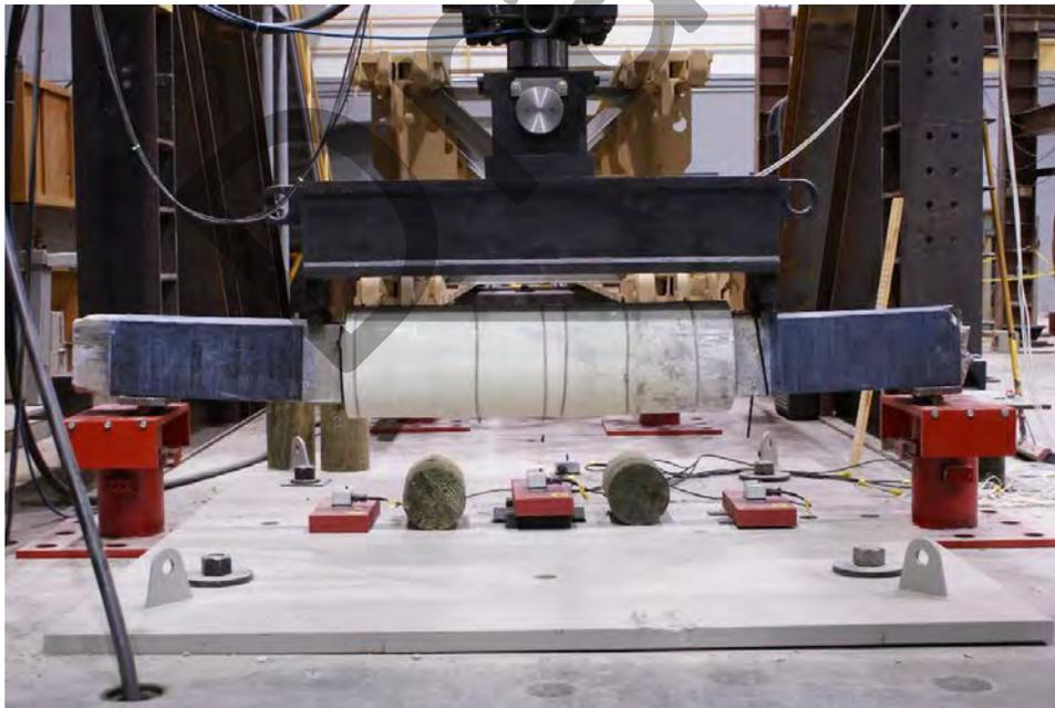
Figure 69. Damaged and dry-retrofitted concrete specimen after flexural testing
