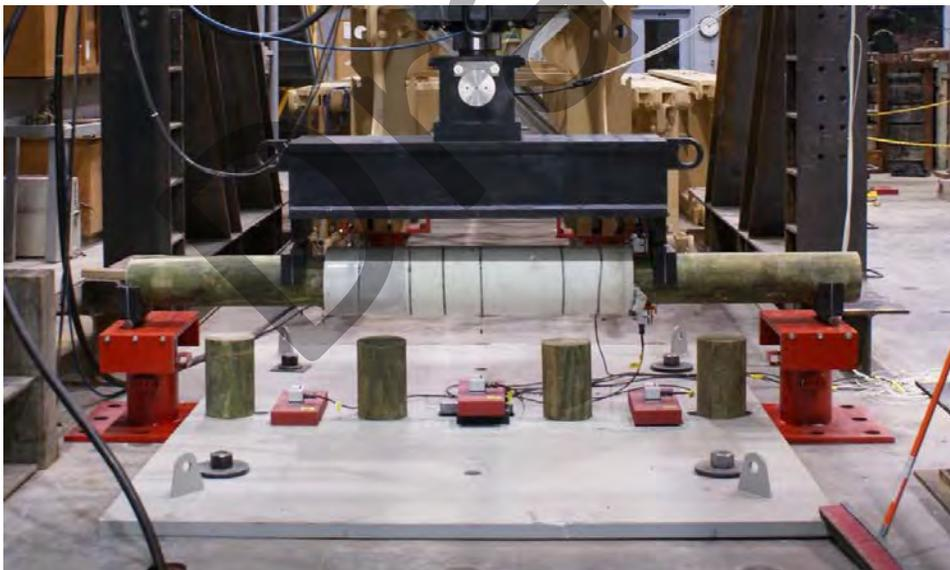
Figure 63. Typical tapered and wet-retrofitted specimen prior to flexural testing
