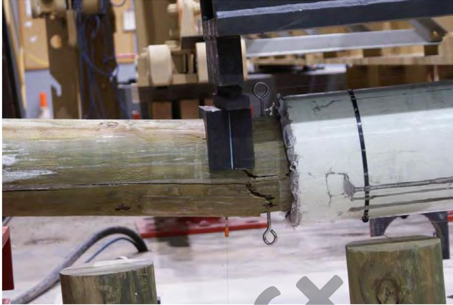
Figure 61. T-RD-2 timber specimen failure after flexural testing
