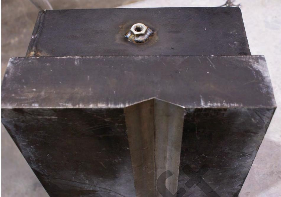
Figure 26: Knife-edge notch in the bottom base plate
