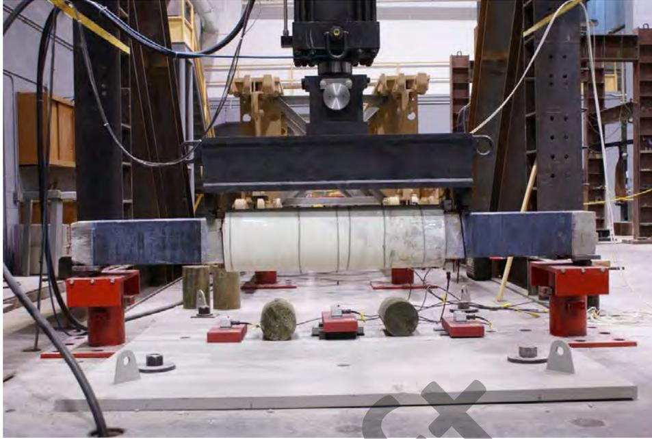
Figure 68. Damaged and dry-retrofitted concrete specimen prior to flexural testing
