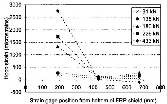
**Fig. 12.** Hoop strain distribution on outer fiber reinforced polymer (FRP) shell at different load levels for repair system B (specimen B2)
