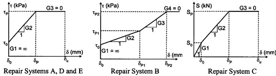
Fig. 13. Simplified model of shear stress (shear force) slip
