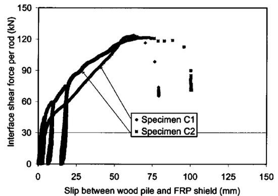
**Fig. 9.** Shear force-slip response for repair system C
