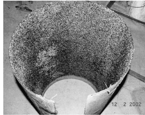
Fig. 2. Polymer concrete coating on interior surface of the fiber reinforced polymer composite shell
