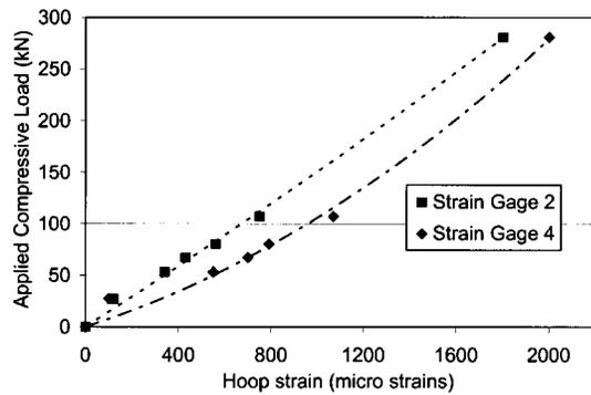
**Fig. 10.** Hoop strain versus compressive load applied at opposite circumferential locations for specimen A1
