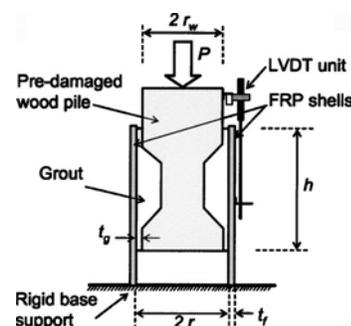
**Fig. 4.** Schematic of test setup for repair system B
