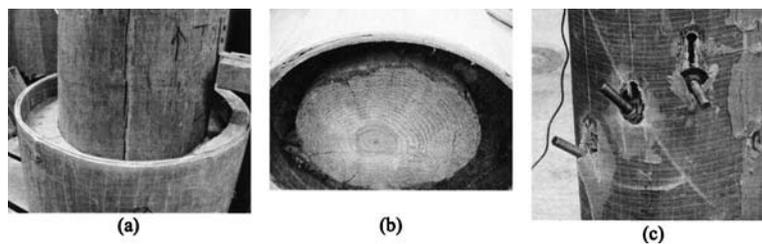
Fig. 6. Typical failure: (a) Interface between the fiber reinforced polymer (FRP) composite shield and cement-based grout; (b) interface between wood pile and cement-based grout; and (c) crushing of FRP composite shield by mechanical connectors
