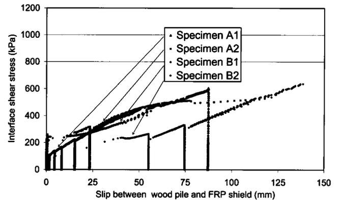
**Fig. 7.** Shear stress-slip response for repair systems A and B
