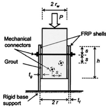
Fig. 5. Schematic of test setup for repair systems C and D
