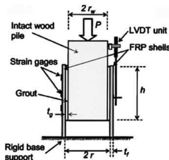
**Fig. 3.** Schematic of test setup for repair systems A and E
