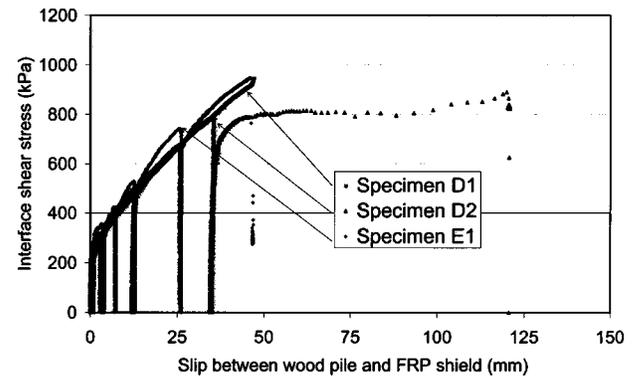
**Fig. 8.** Shear stress-slip response for repair systems D and E
