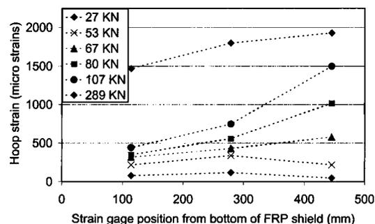
**Fig. 11.** Hoop strain distribution on outer fiber reinforced polymer (FRP) shell at different load levels for repair system A (specimen A1)
